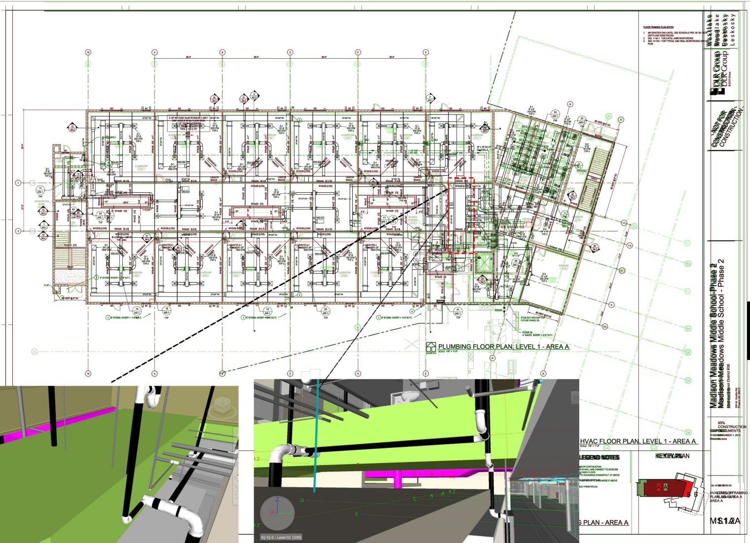
55X24 duct clashing with the framing and multiple vertical and horizontal pipes, not enough space to move it anywhere.
